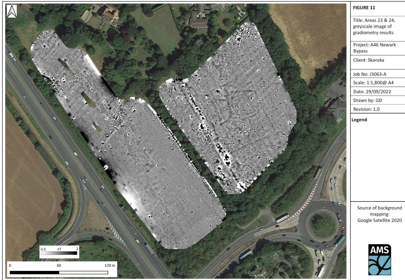
Figure 11: Areas 23 & 24, greyscale image of gradiometry results
