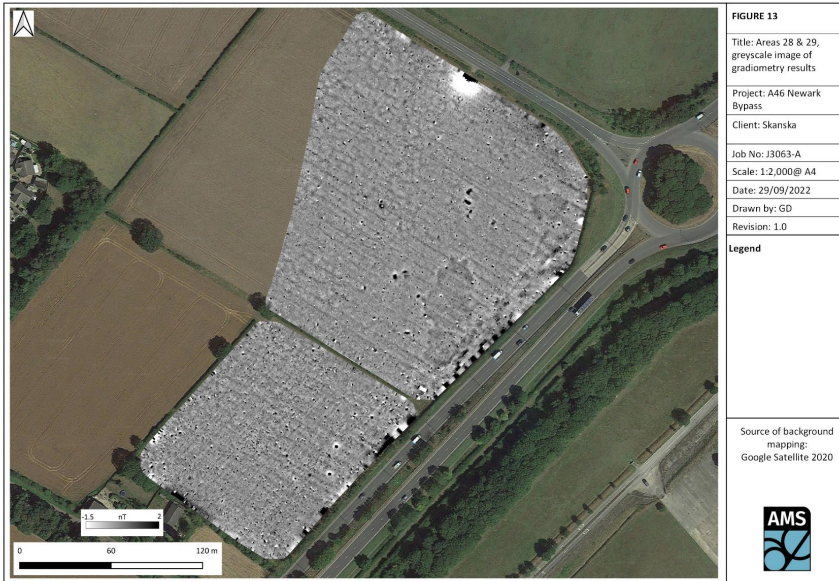
Figure 13: Areas 28 & 29, greyscale image of gradiometry results
