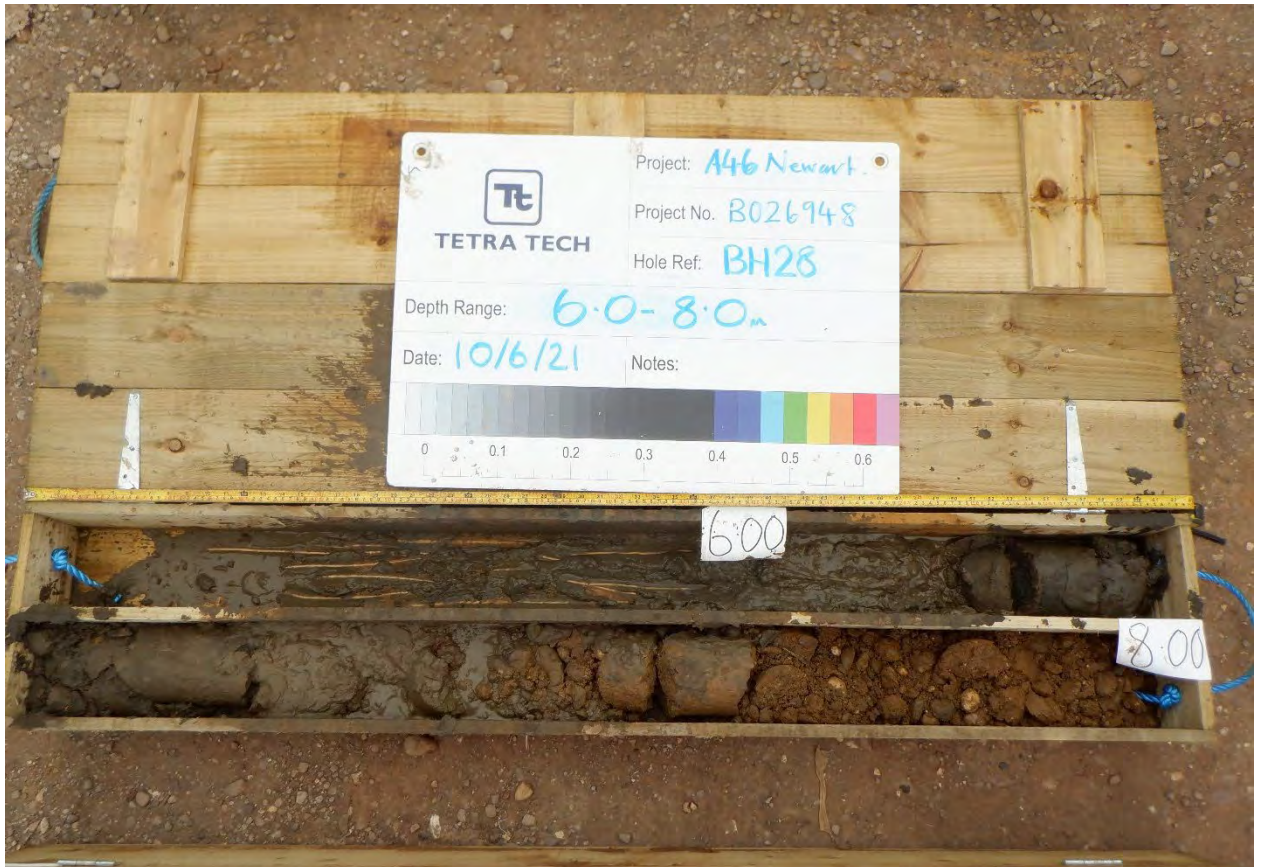
Plate 6: BH28 6.00-8.00m BGL (Not sampled due to poor recovery / sand dominated).
