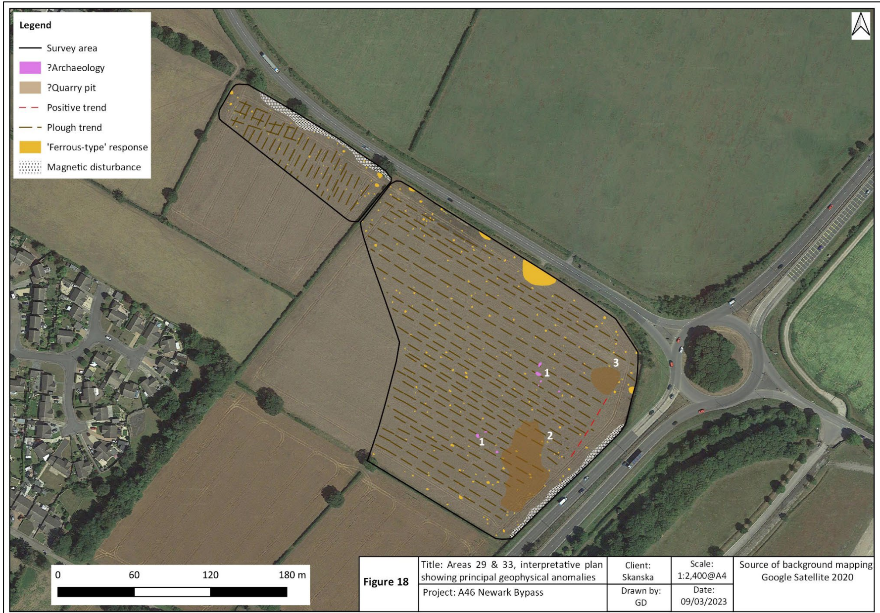
Figure 18: Areas 29 & 33, interpretative plan showing geophysical anomalies.
