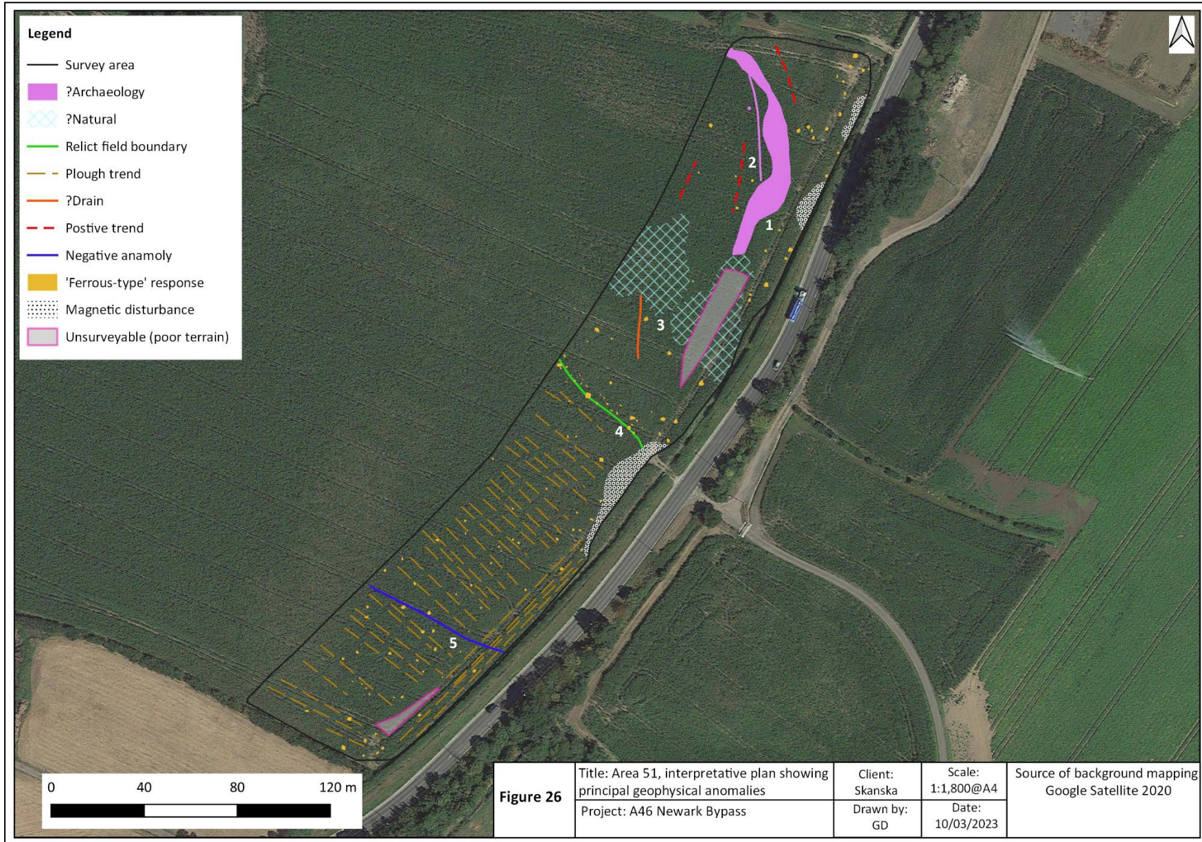
Figure 26: Area 51, interpretative plan showing principal geophysical anomalies.
