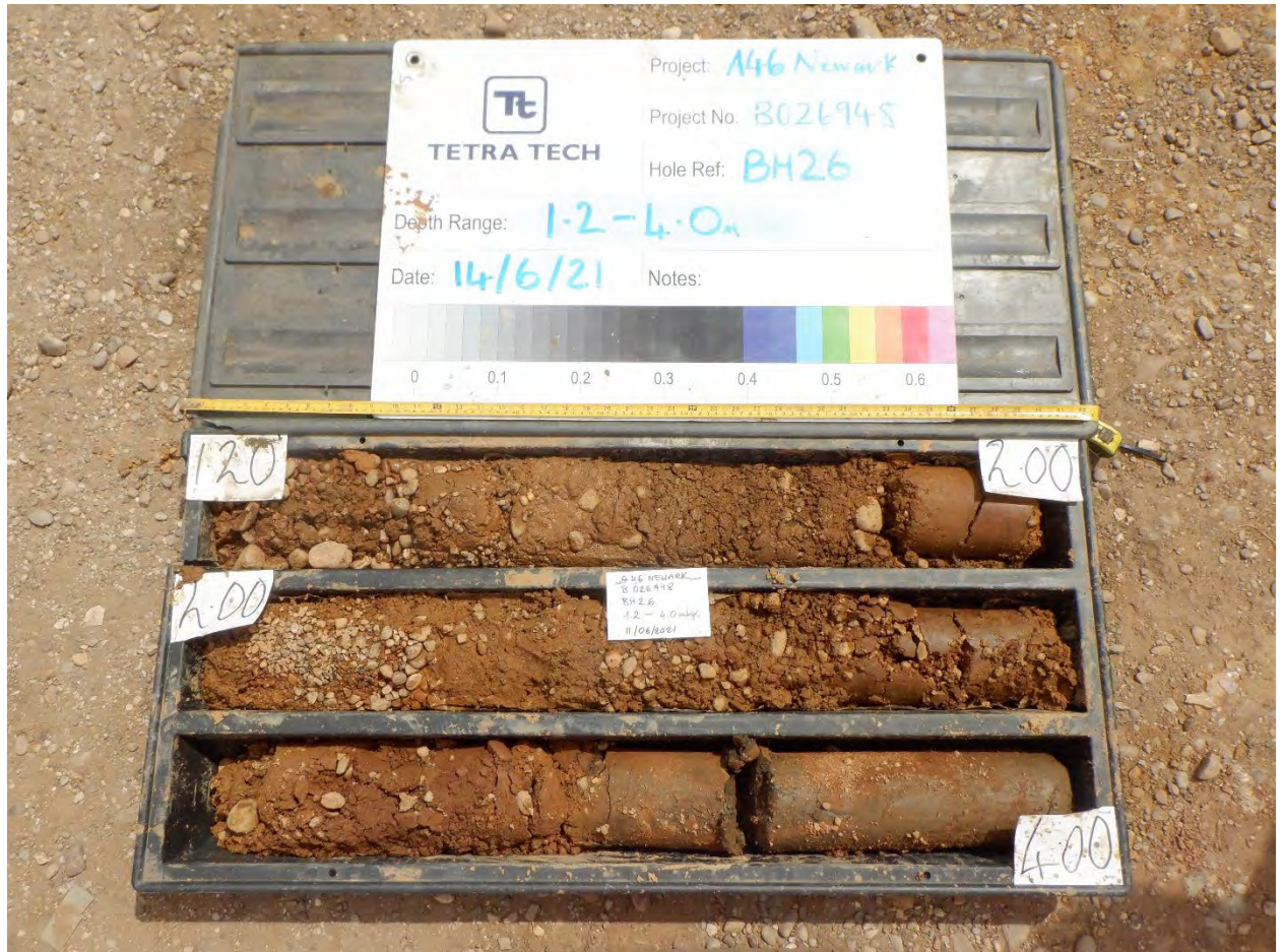
Plate 3: BH26: 1.20-4.00m BGL (Not sampled due to desiccation of organics; example of organic deposit likely truncated by the construction of the embankment)
