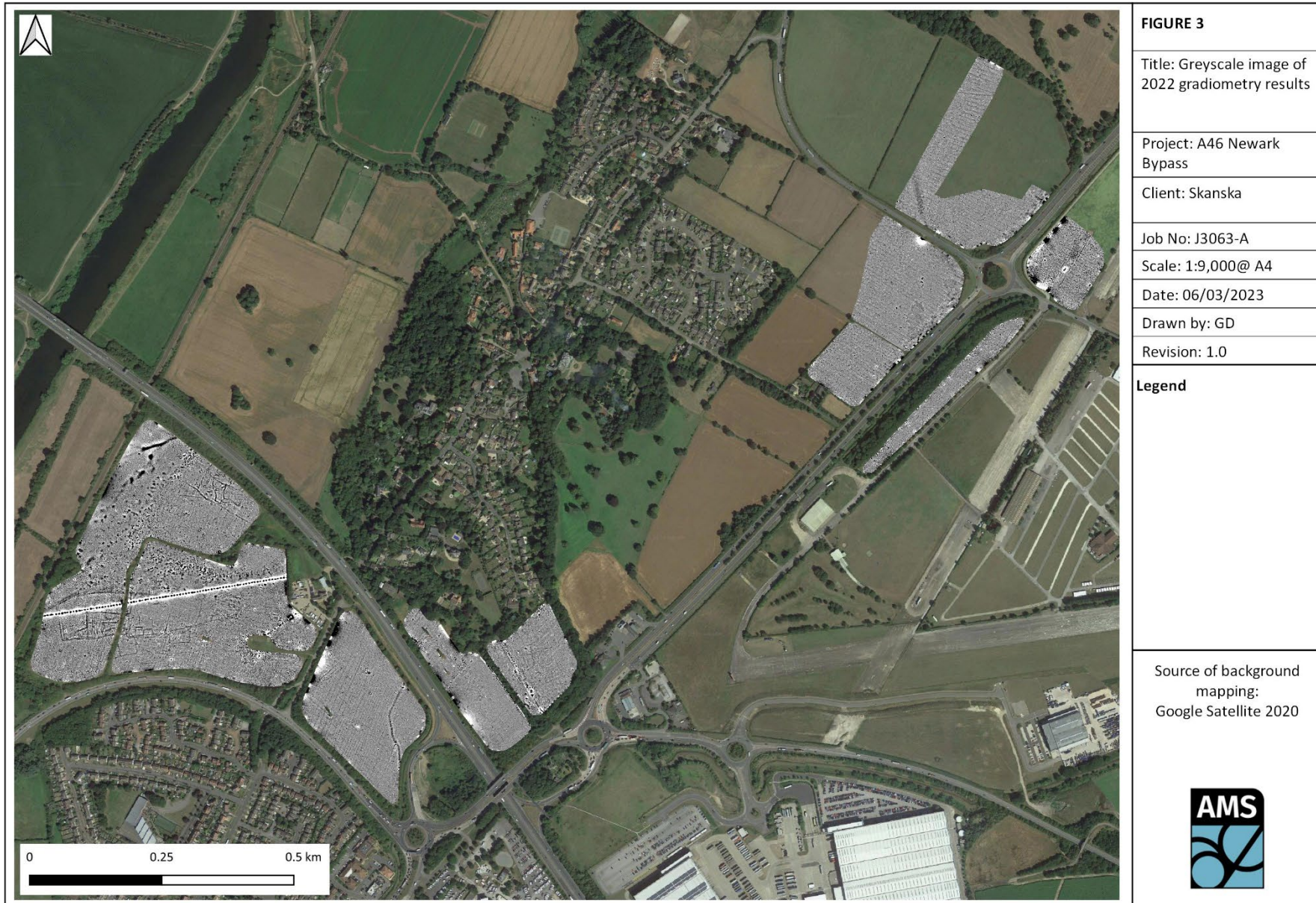
Figure 3: Greyscale image of 2022 gradiometry results (Areas 20–24 & 28–32).
