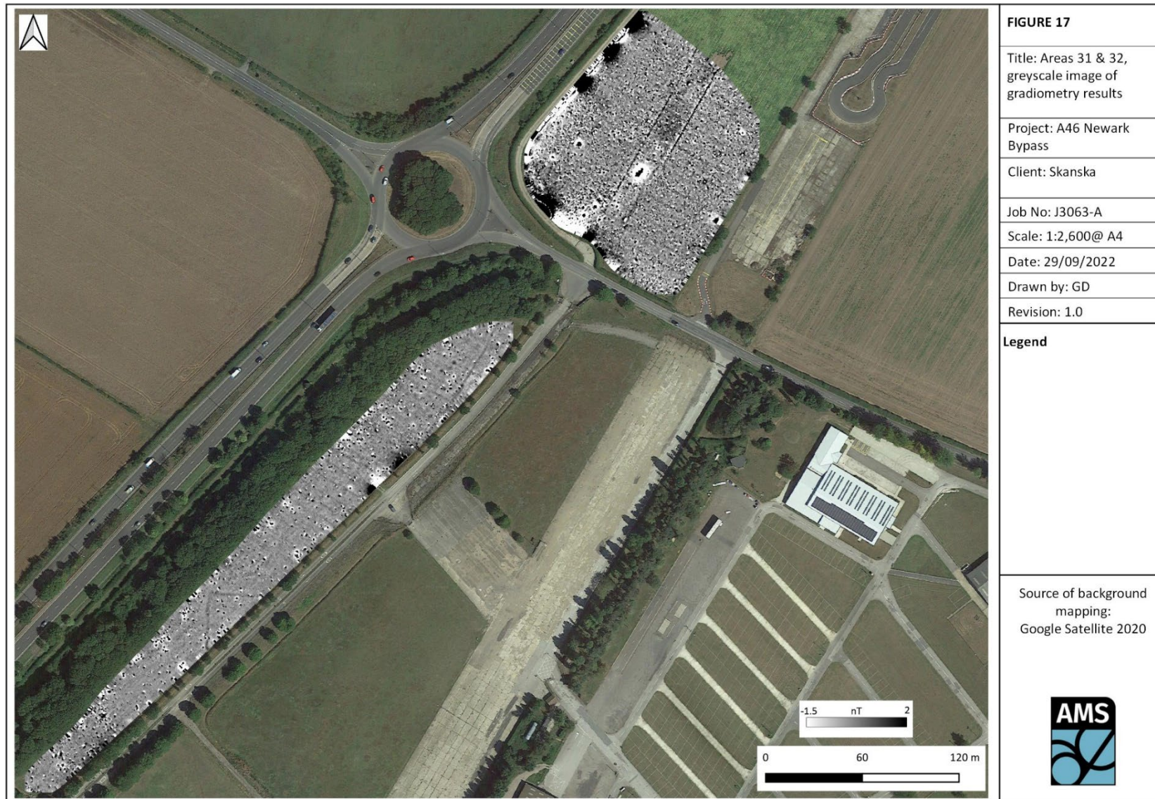
Figure 17: Areas 31 & 32, greyscale image of gradiometry results
