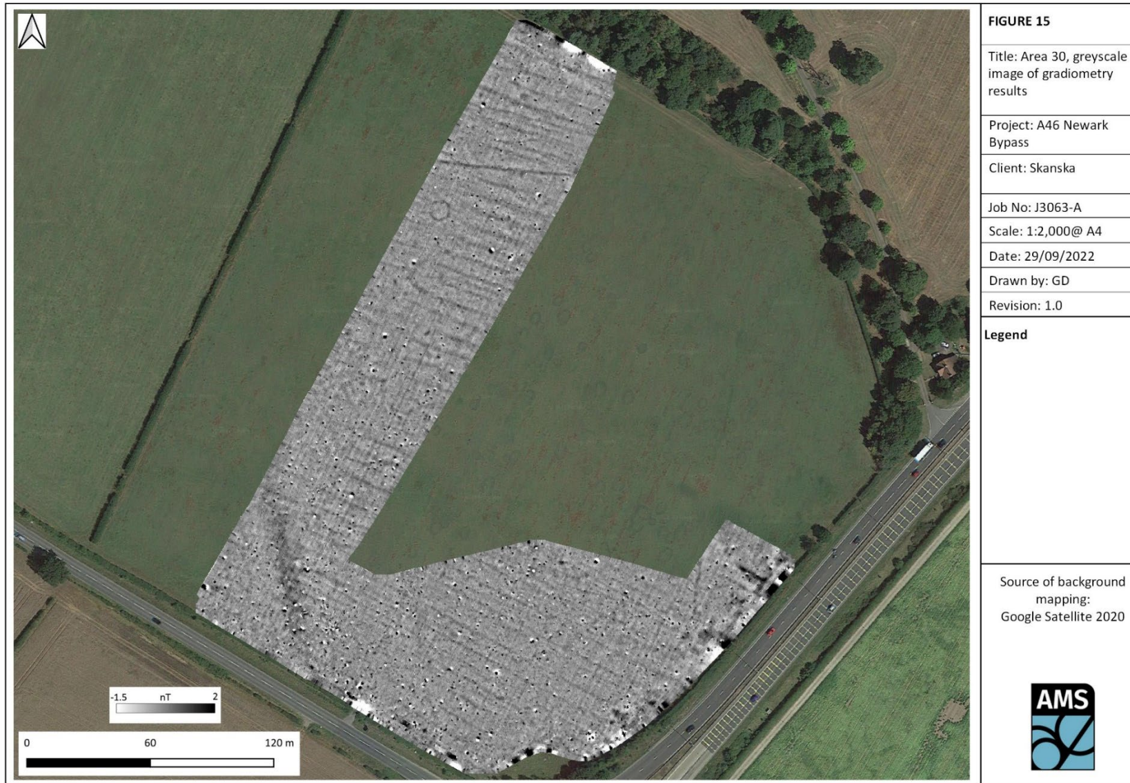
Figure 15: Area 30, greyscale image of gradiometry results
