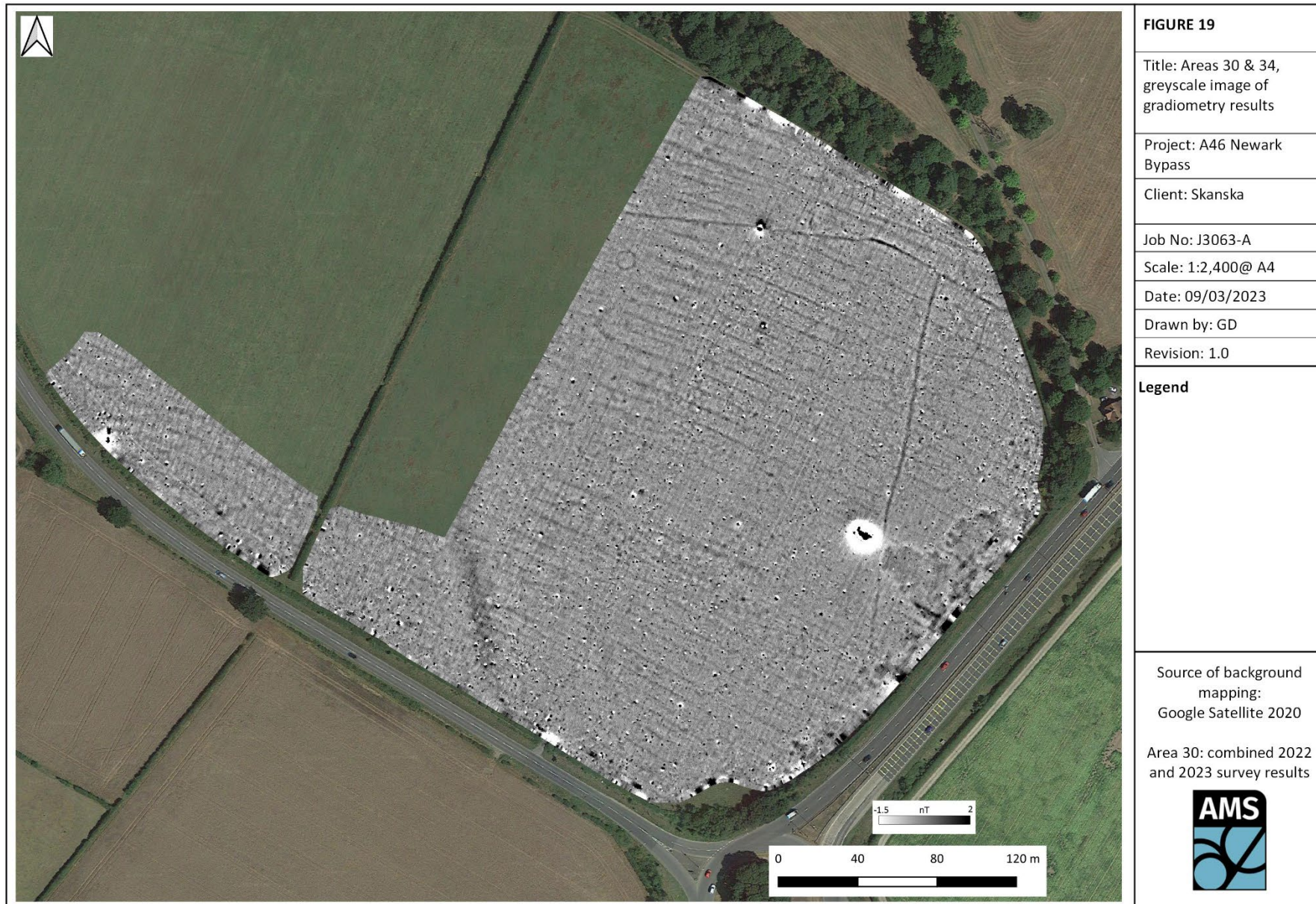
Figure 19: Areas 30 & 34, greyscale image of gradiometry results.
