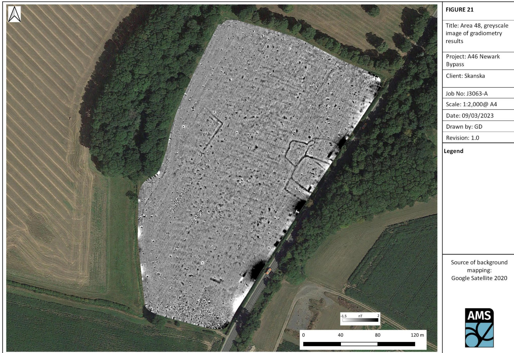
Figure 21: Area 48, greyscale image of gradiometry results.
