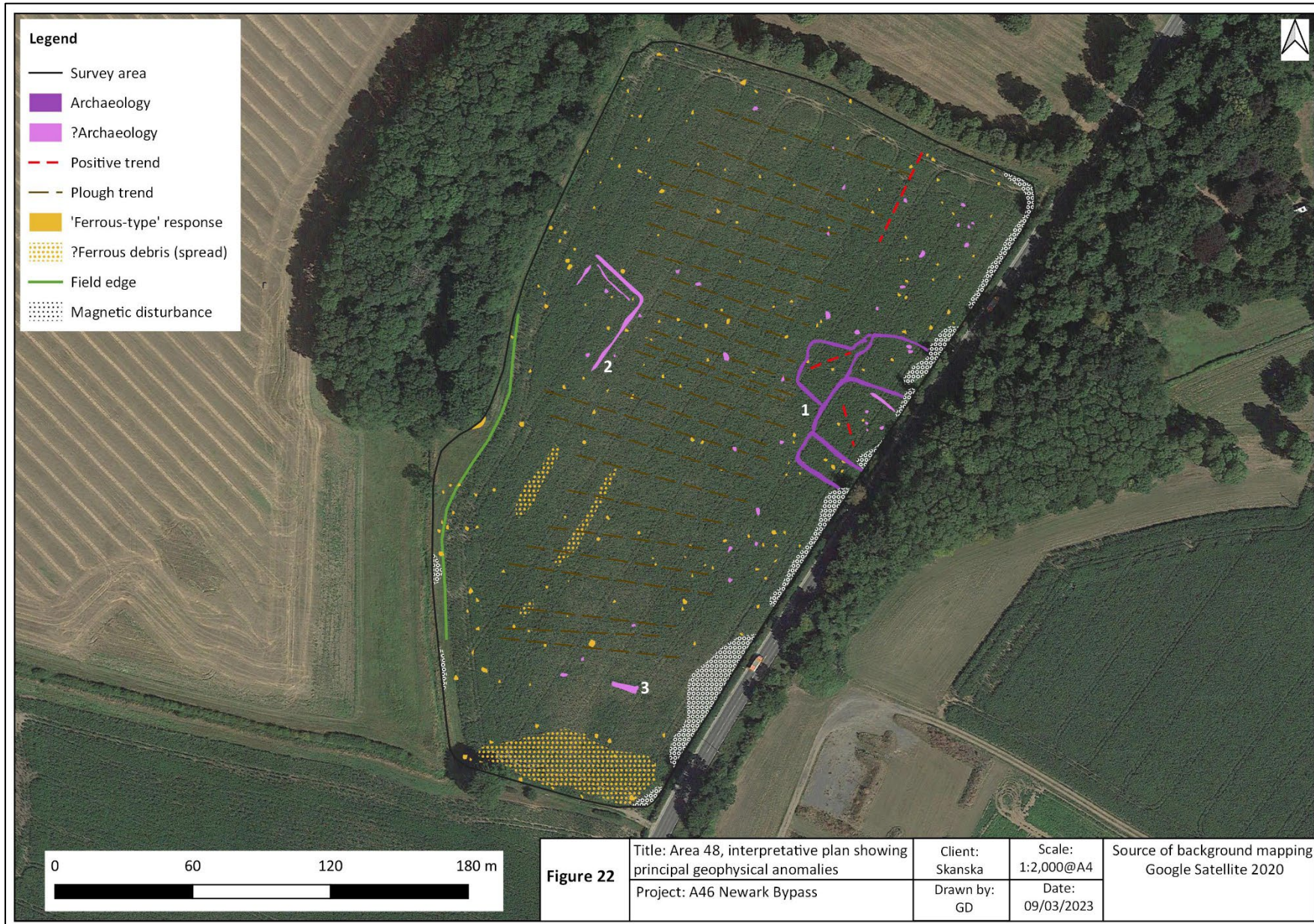
Figure 22: Area 48, interpretative plan showing principal geophysical anomalies.
