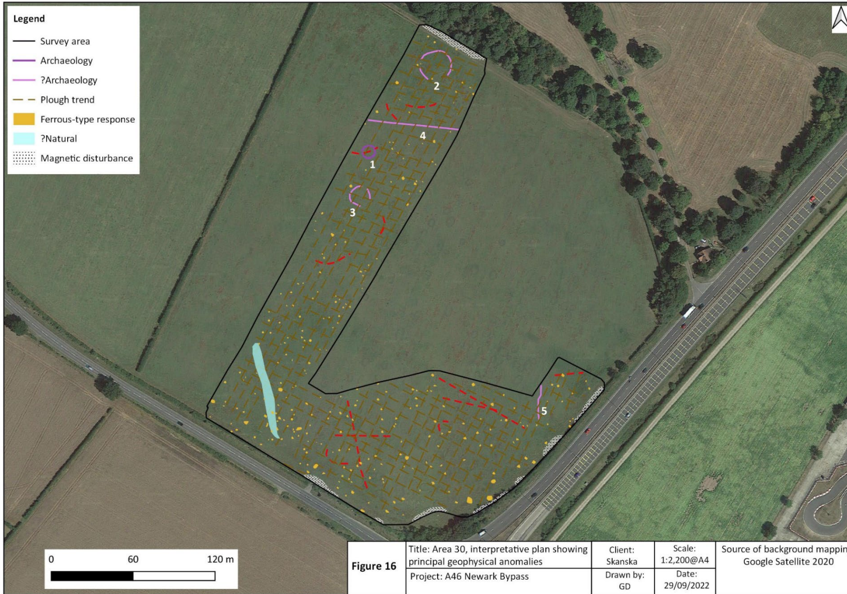
Figure 16: Area 30, interpretative plan showing principal geophysical anomalies
