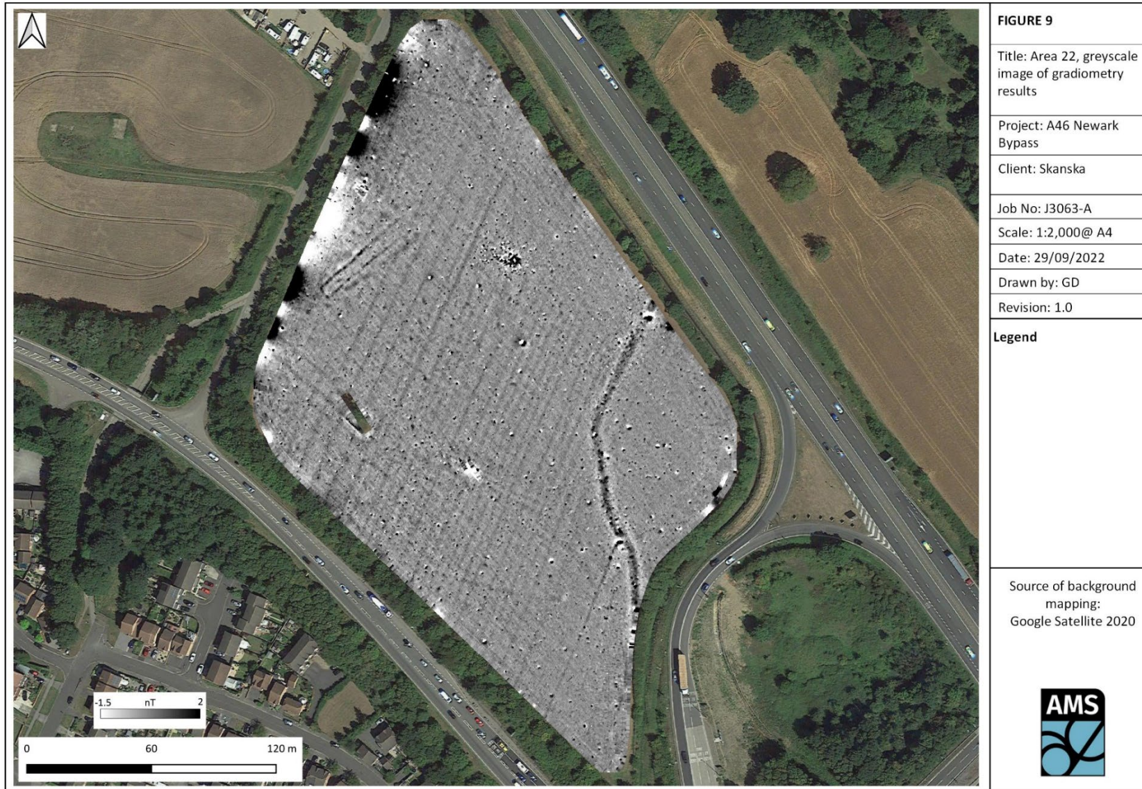
Figure 9: Area 22, greyscale image of gradiometry results
