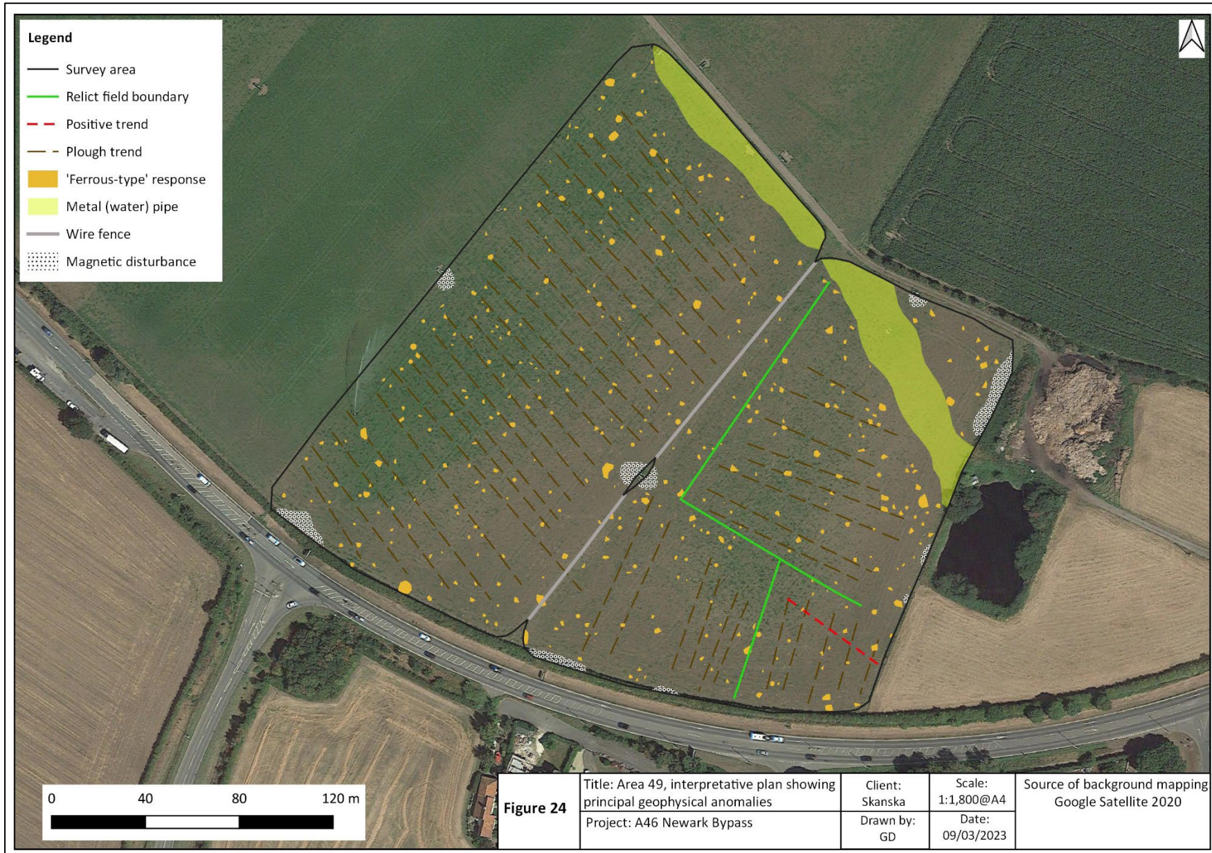
Figure 24: Area 49, interpretative plan showing principal geophysical anomalies.
