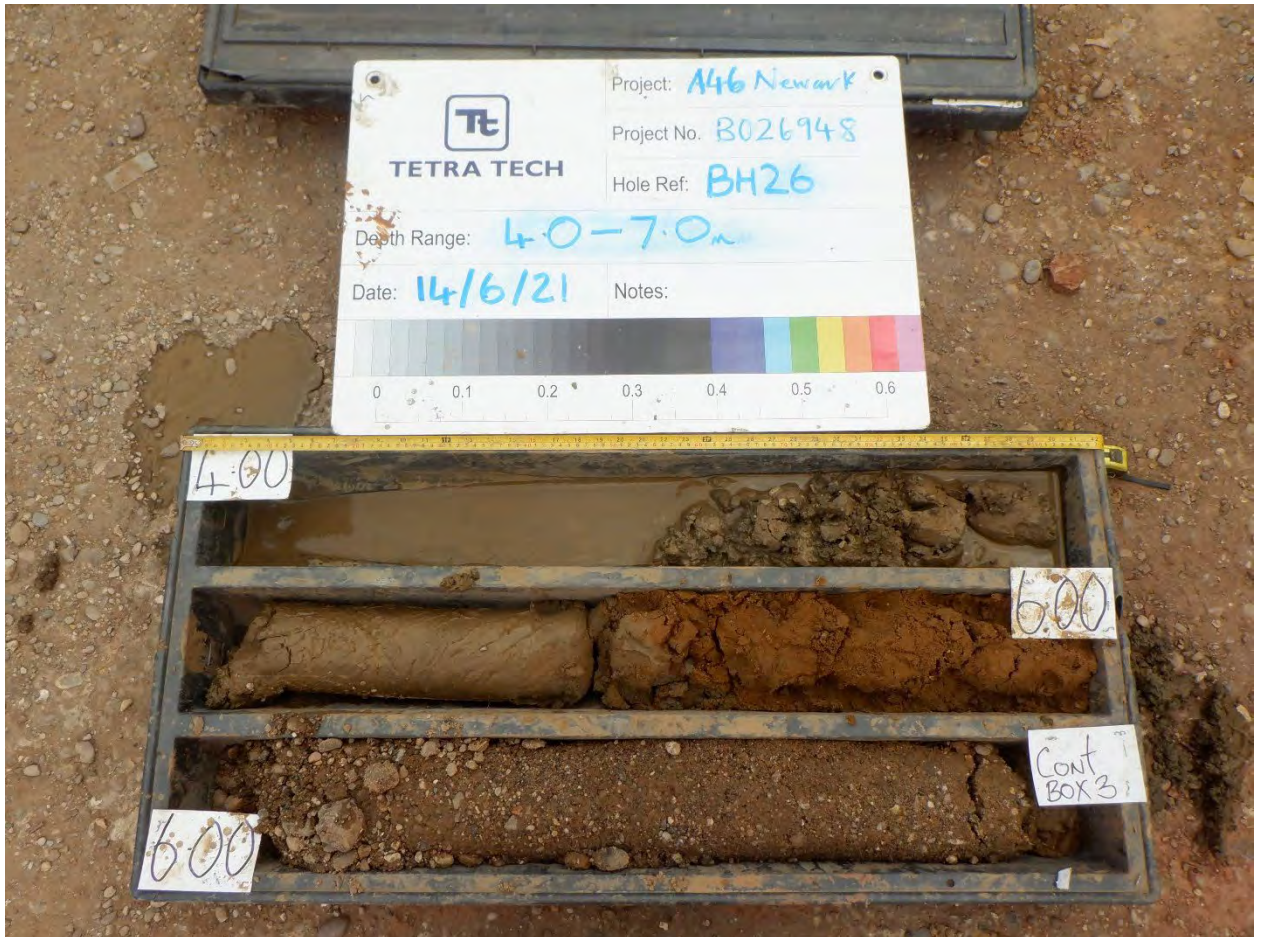
Plate 4: BH26: 4.00-7.00m BGL (not sampled due to poor recovery; ex-situ oxidization)
